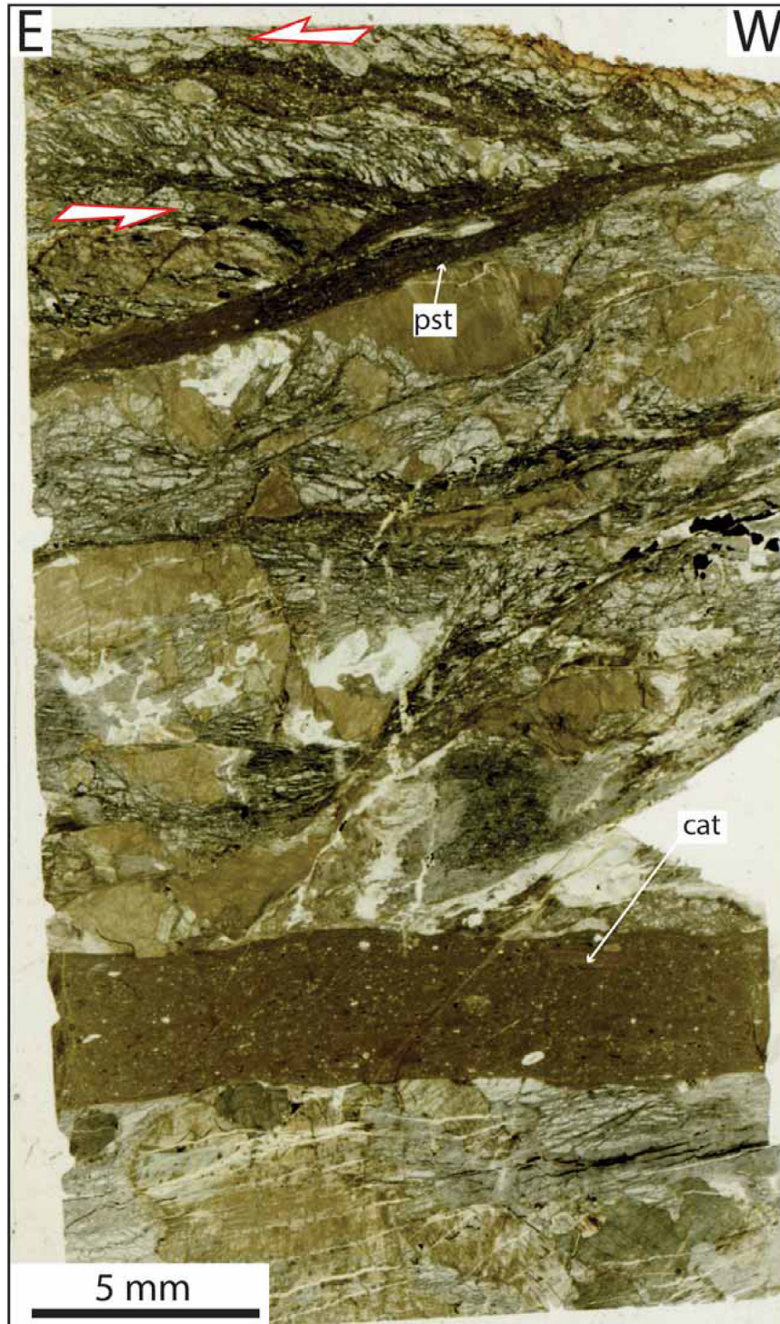
Fig. 4. Scanner image of a thin section showing a cataclastic peridotite crossed by a pseudotachylyte fault vein (pst) and by a cataclasite layer (cat) formed at the expense of a pre-existing pseudotachylyte fault vein.
